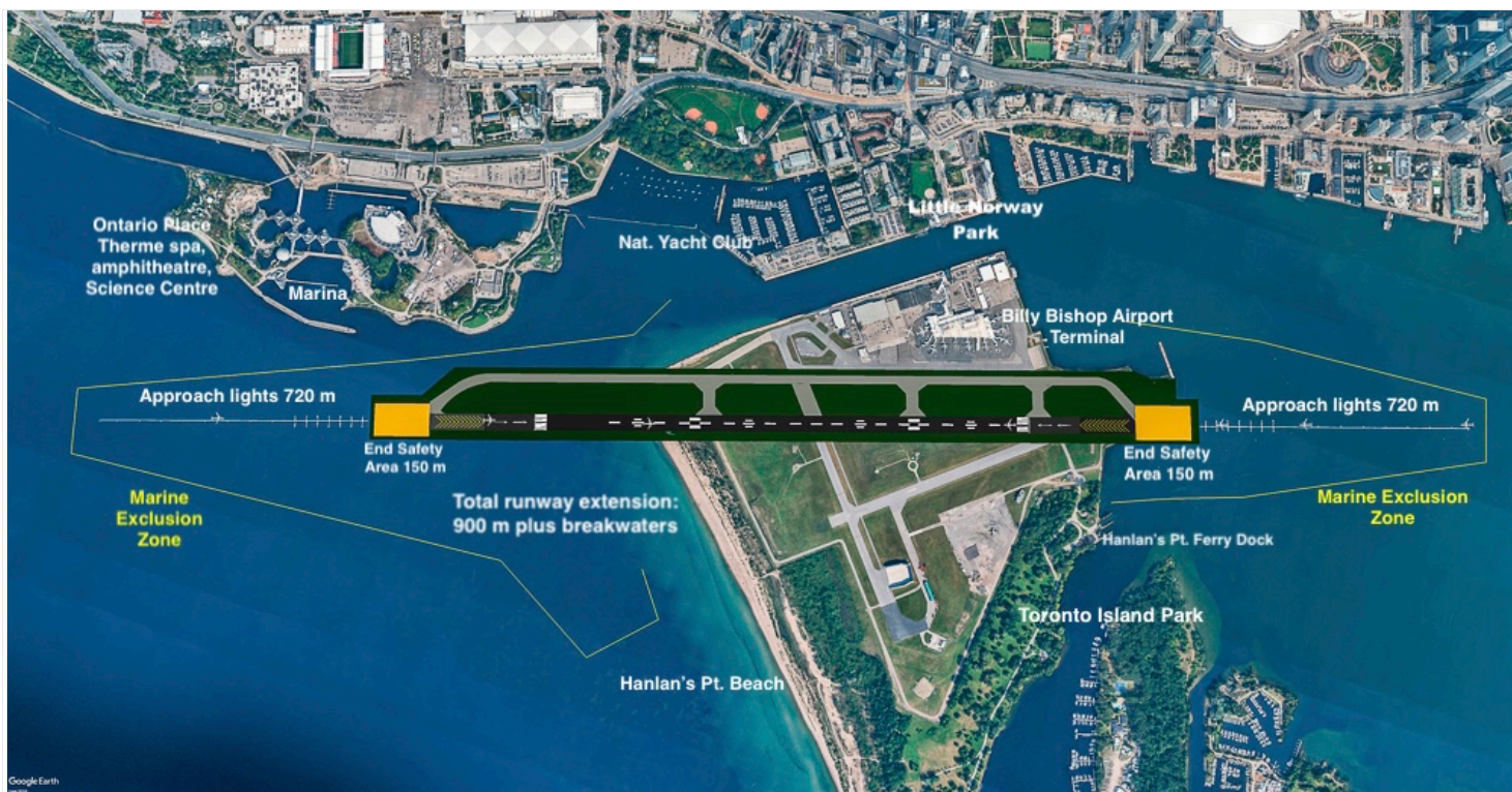
Based on existing information - extended runway and approach lights as anticipated by Spacing magazine online 9
